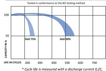
le life is measured with a discharge current 0,2C, charged 16h and rest capacity of 2/3 Cn
