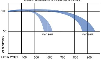
\* Cycle life is measured with a discharge current 0,2C, charged 16h and rest capacity of 2/3 Cn
